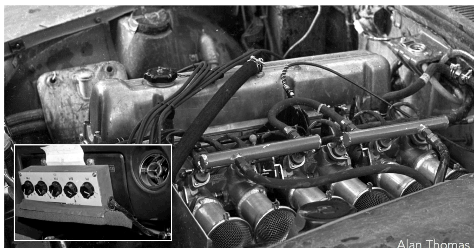
5. 1973 LR24 Works engine with ECGI and Navigator control panel (inset)
